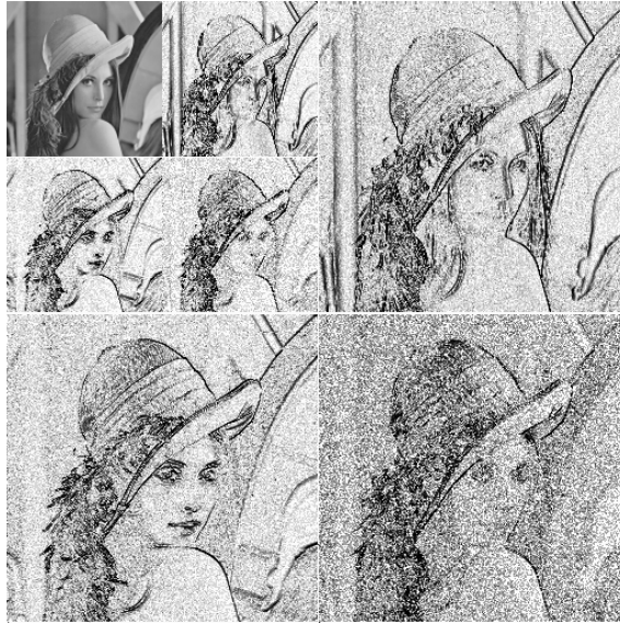
Figure 3.8: Wavelet transformation example: enhanced detail bands
