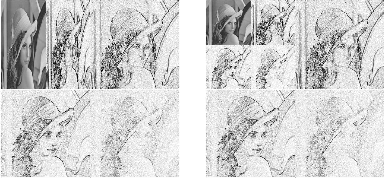
Figure 3.7: Wavelet transformation example: next coarser level
