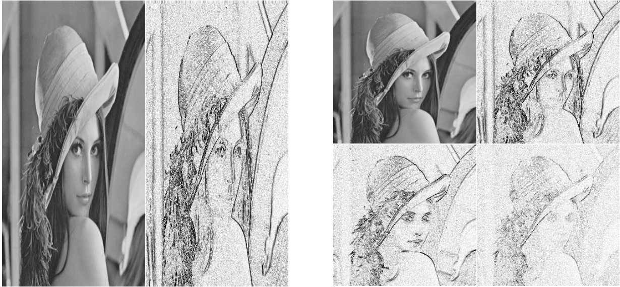
Figure 3.6: Wavelet transformation example: finest level
